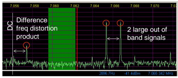
Real life example of op-amp with *moderate distortion specs* operating *at low voltage* and using *too much gain*
