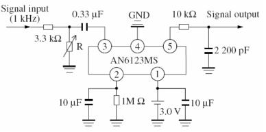
AN6123 typically used as an AGC stage in a cordless telephone
