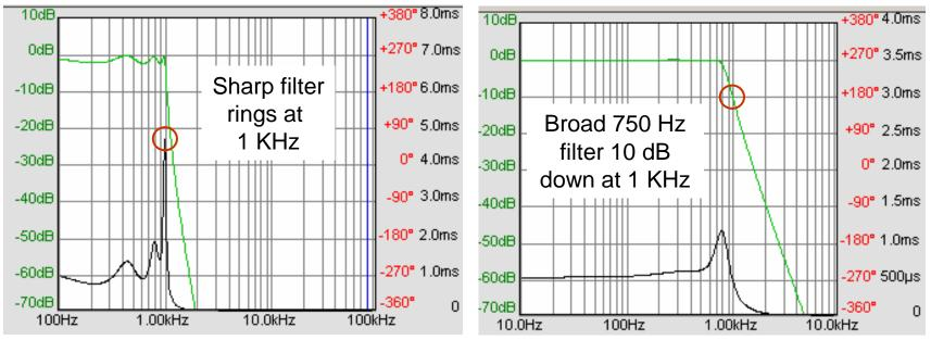
Broad 750 Hz "post filter" used to clean up high Q "ringing" at 1 KHz Filter pair totals 110 dB down at 2 KHz – Very high performance indeed! Trick used in NC2030 – Main R/C filter + very sharp SCAF headphone "clean up" filter 10/18/08 Receiver Audio Filtering Dan Tayloe, NTVE
